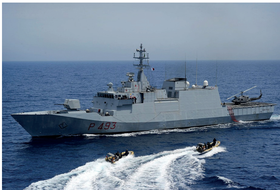
Figure 4. The 1520 tons ITS Commandante Foscari patrol vessel is a part of the Italian Green Fleet Program propelled by “Green Diesel” acquired from vegetable oils and tallow. This fuel conforms to F76 NATO navy fuel standard. [19]
