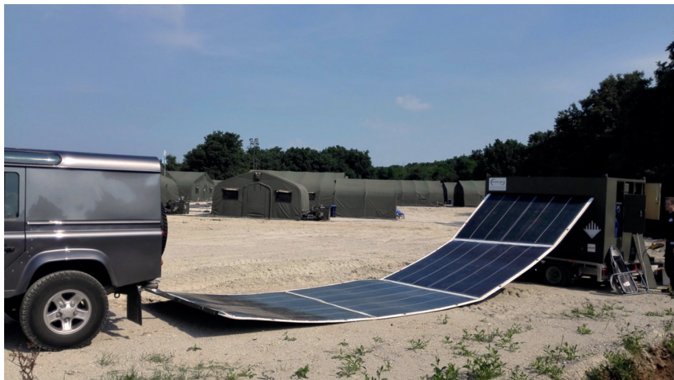
Figure 9. The theory of the British Renovagen is very special and compact. The trailer contains the retractable solar-carpet and the inverters. The tractor Land Rover helps the quick deploy.
